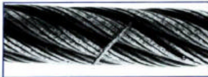
Severe abrasion, broken wire
