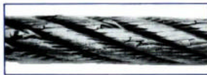
Severe abrasion, peening, broken wires
